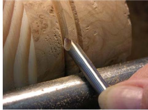
Correct Tool Movement: The movement of simultaneously rolling the tool and lowering the handle to produce a slicing cut is essential.
