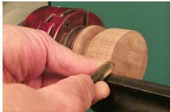
7. Face off the top with a 3/8" spindle gouge or skew chisel.
