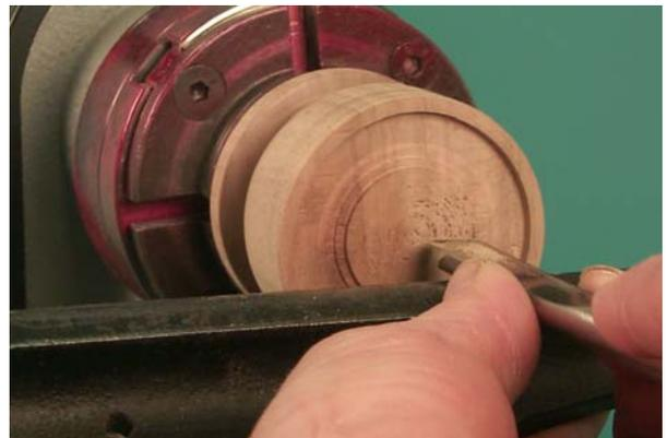
12. Remember to check your depth often so that you do not risk going through the bottom when you later reverse turn the bottom. You also need to check the wall thickness to insure that it is even.
