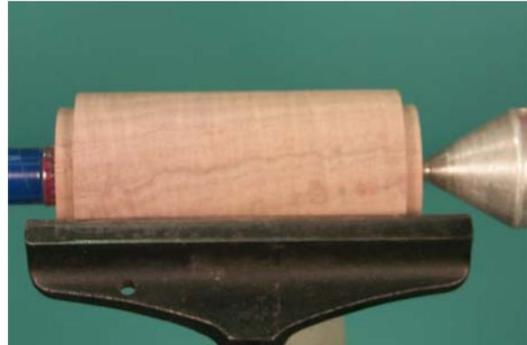
4. Measure the length of box, making sure to leave room at the ends for the 1/4" tenon and allowing clearance for the tool when shaping top and bottom in the chuck.
