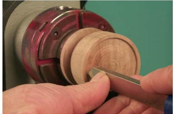
9. Begin hollowing using a spindle gouge or hollowing tool.
